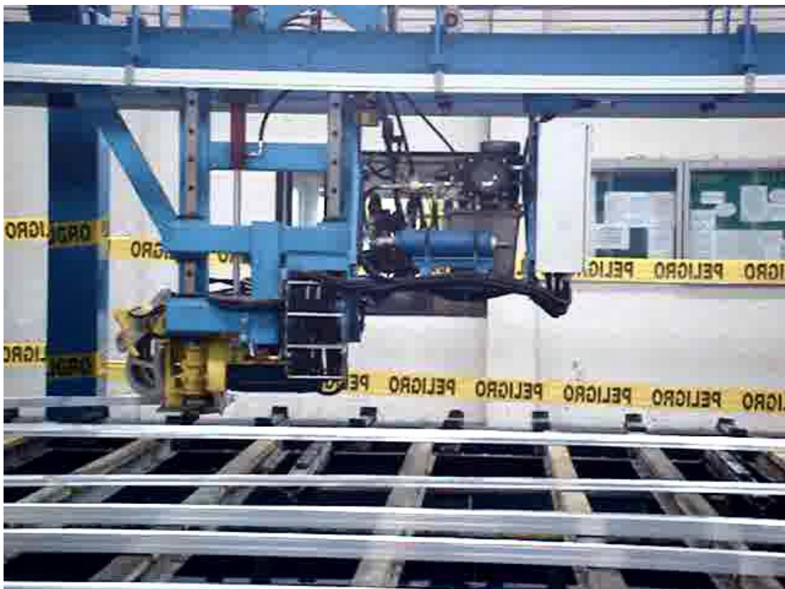
(2) 雙牽引機，左車頭牽引。 Double Puller, Left Puller Head pulling.
