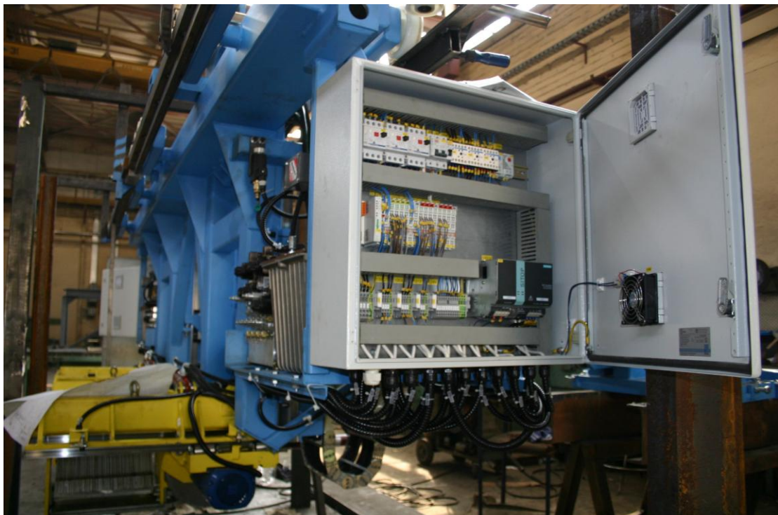
(2) 雙牽引機，車頭 PLC 電控箱。Double Puller, Puller Head PLC Control Panel.
